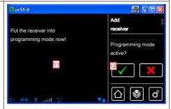
13 In addition to the information on the screen saying that the programming has been completed successfully, many receivers also confirm correct programming. This is often done by "clicking" at motors, or by flashing the status LED at the receiver. The manual for the receiver concerned will tell you whether the receiver you are programming provides confirmation, and if so, how.
