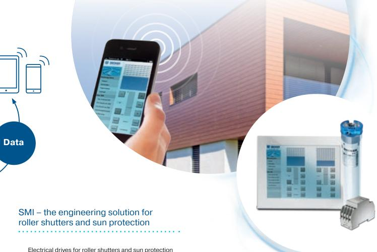
Electrical drives for roller shutters and sun protection installations can also be integrated into the KNX bus system with the standardised SMI (Standard Motor Interface).
